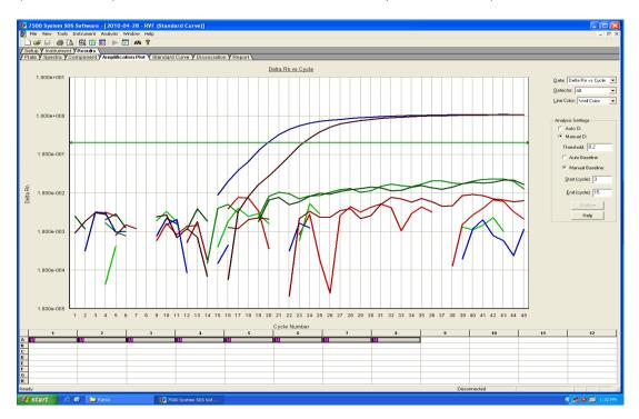
**Figure (1):** The real-time detection of the specific PCR products by fluorescence (y axis) (F1 detection wavelength or F1/F2 ratio) dependent on the PCR cycle number (x axis).
